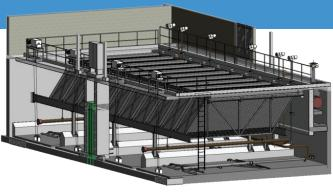
←↑ Our new inclined plate settlers are custom built into the basins originally constructed for the old clarifiers. The first unit was placed into service in July of 2024. Plant staff reported an immediate improvement in pre-treated water quality and zero temperature-induced process upsets. The improved pre-treatment water quality has led to better filtered water quality, which is central to compliance with the Safe Drinking Water Act.
