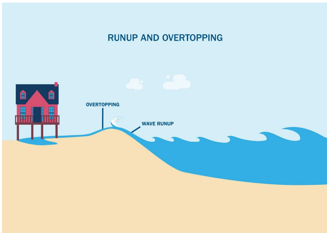
Figure 5b: Wave Overtopping Schematic
